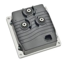
**1216 motor controllers** are programmable, a low cost, high performance solution for pump motor control applications including scissor lifts, lift trucks, mobile booms, or any pumping application where 24-volt, series motor, speed control is employed. 1216 controller is a programmable motor controller, it can program the controller parameters by handheld programmer for different generation Genie scissor lift.
